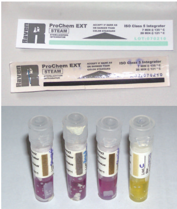
Figure 16: Steam integrators (top) and self-contained biological indicators (SCBIs) (bottom) (Source: Stringer, HECAF 360)
